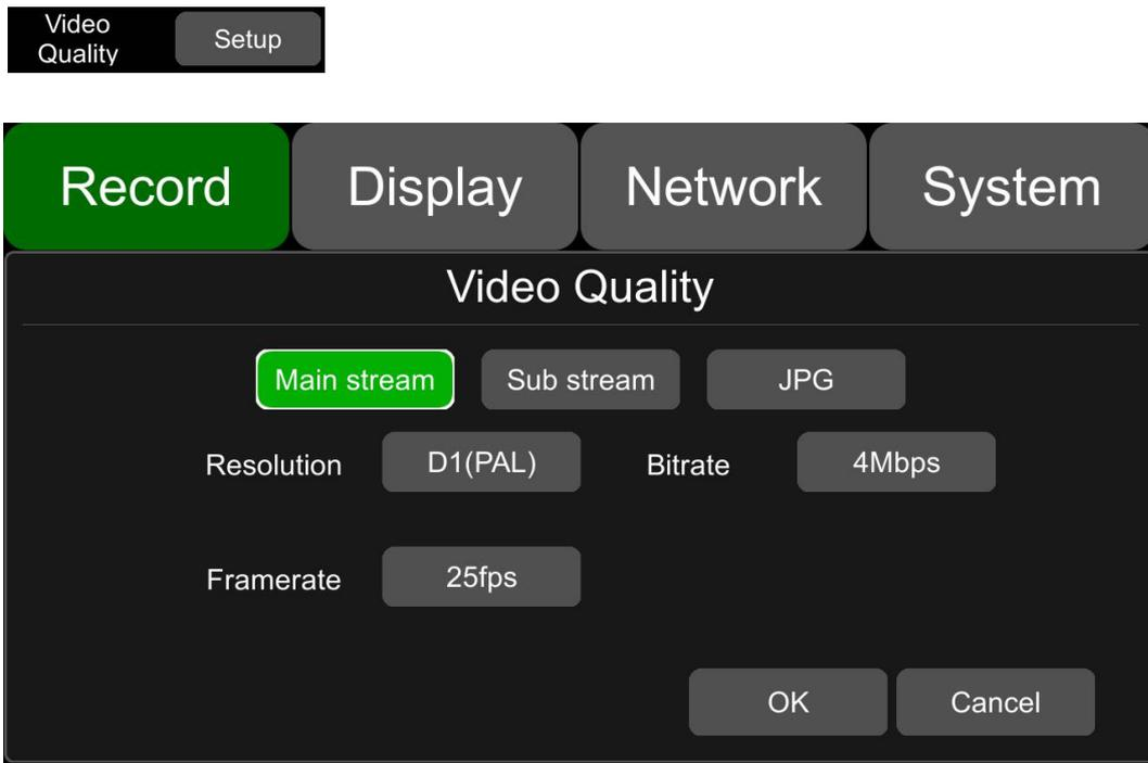
The main stream is used for video storage. The sub stream is used for network transmission.
