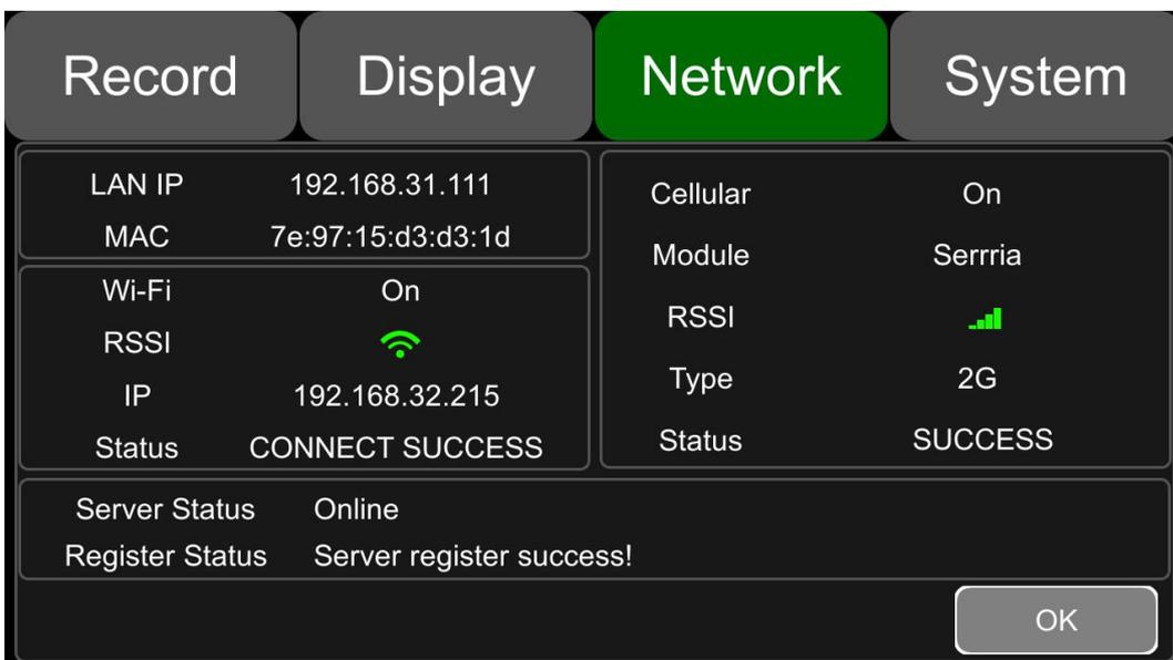
LAN IP: The static IP set on Network-LAN page or the dynamic IP obtained automatically.
