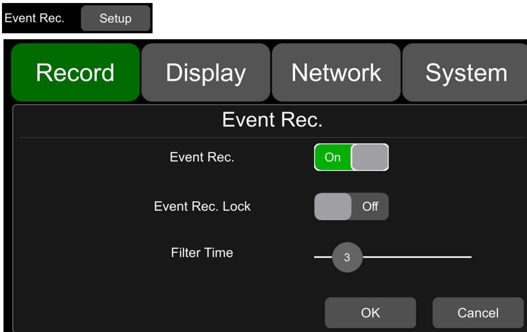
**Event Rec.:** Event recording refers to the alarm recording triggered by events including motion detection, G-force, alarm 1 ~ 6, panic button, radar detection , inappropriate drivers' action warning , driving safety risk and over speed. If the Event Rec is set to ON and corresponding alarm parameters are set, event recording will be activated when the events above are triggered. If the Event Rec is set to OFF, event recording will not be activated even if an alarm is triggered.
