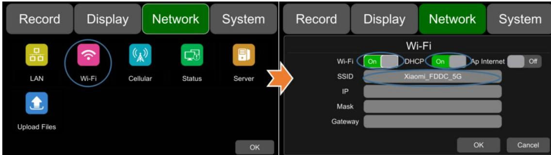
Step 4: Touch SSID sub-menu to select the hotspot and input the password.
