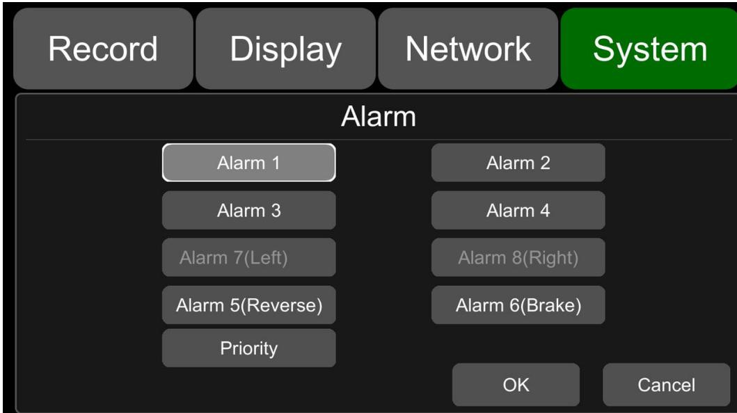
**Alarm 1~Alarm 4:** Customized alarm recording.
