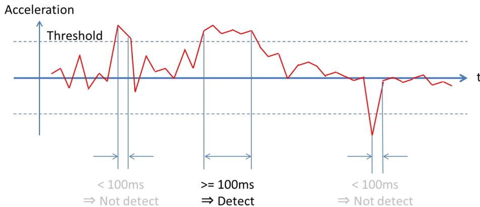
Pic 1.1 Principle of G-force Alarm Triggering Detection
