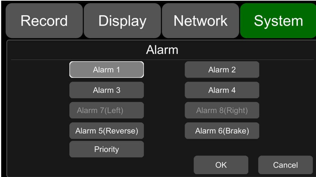
2) Alarm output 1 and alarm output 2 are 12V by default, which can be used as a trigger and working together with alarm inputs. You can also set up the BUZZER as one output.
