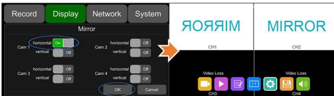
Vertical: set to “ON”, the corresponding channel flips vertically; set to “OFF”, the corresponding channel displays normally, without flipping.
