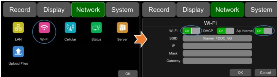
Step 3: Search and connect to the Wi-Fi hotspot of the DVR with other mobile devices. The SSID name of the hotspot is prefixed with "WFD-" and followed by the serial number of the device. "WFD-" default password is ap12345678.
