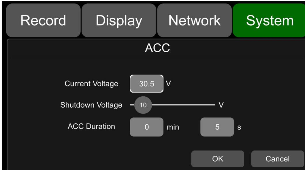
The default configuration of "Shutdown Voltage" and "ACC Duration" is shown above.
